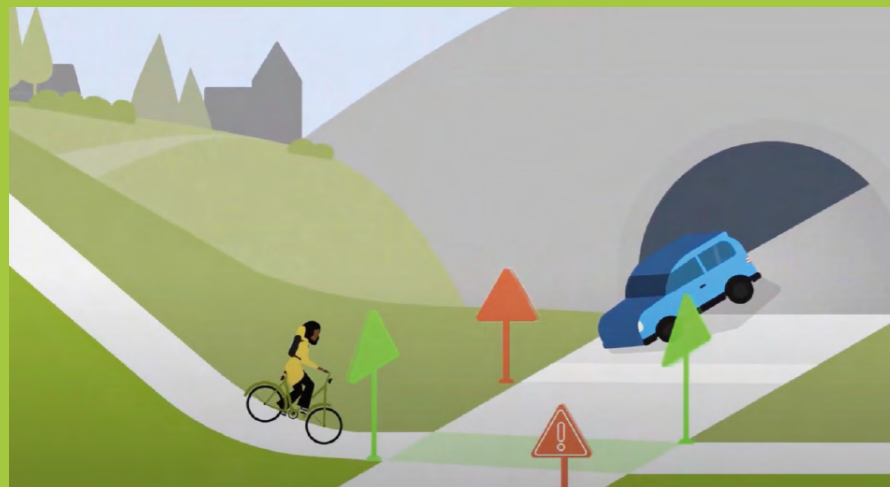
Figure 5.2: Extended green for cyclists cycling downhill in Aarhus
